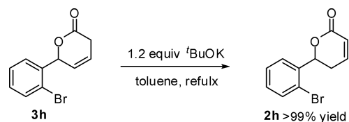
Scheme 2 Conversion 3,6-dihydro-2 H -pyran-2-one to 5,6-dihydro-2 H -pyran-2-one.
